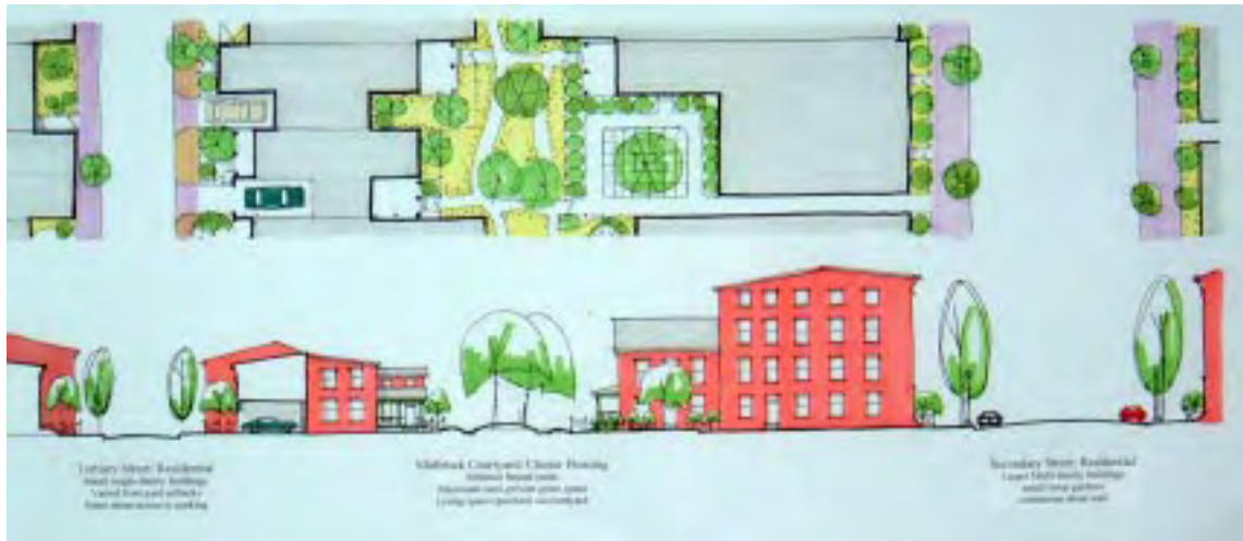
Figure 51: Enhance residential spaces with an urban landscape of outdoor private spaces. Decks, balconies, and porches provide residents with much needed private space that also function to enliven and safeguard the semi-public space of courtyards, and the public space of alleys and streets. Privately maintained urban landscapes, including window boxes and stoop entry gardens, provide both beauty and a sense of ownership for the environment.
